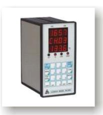
In a process control environment, many events like Solenoid operations, relay operations, Alarms etc. occur and it is important to log the sequence of these events. Event logger accepts digital / ac inputs and keeps a track of such events.
