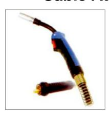
Cable Attached Metal Inert Gas Torch requires 250 Ampere current to operate efficiently and is available in air-gas cooled version. The Metal Inert Gas Torch is offered in different lengths such as 3m, 4m and 5m. The Metal Inert Gas Torch that comes under MT-24KD-AB model is attached with a cable surface area of 25mm². Cable Attached Metal Inert Gas Torch is extensively used as a welding tool in different industries.
