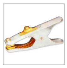
Steel made Earth/ Ground Clamp is widely used for welding and construction sectors. The Earth/ Ground Clamp is made using quality grade hot dip galvanized steel sheet which ensures durability of use along with long lasting trouble free service. The Earth/ Ground Clamp is available under Croco series of model number ECN60. Steel made Earth/ Ground Clamp is designed with double braided copper shunt.
