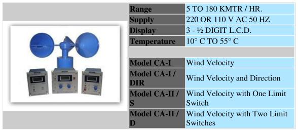
Three conical beaded edged cups 127 mm. In diameters, attached by arms to a central boss drive a vertical spindle at a rotary speed proportional to the air velocity. (dimensions confirming to is 5912: 1970)
