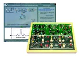
ACT-01 forms the heart of the system, generating all necessary signals for performing various experiments in Analog Communication, which includes all modulating and carrier signals.
