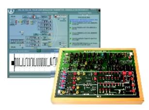
This kit provides two-channel Time Division Multiplexed Pulse Code Modulation in none, even, odd & hamming parity format. It enables students to learn the basics of timing synchronization between the transmitter and receiver. PCM receiver is a separate kit.
