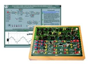
This kit facilitates students to study concepts of Delta Modulation techniques. It facilitates students to examine Delta, Sigma Delta & Adaptive Delta & CVSD Modulation and Demodulation.
