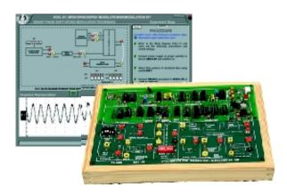
This kit is designed to provide knowledge of advance digital modulation techniques like BPSK, DPSK & DEPSK.
