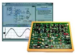
FCL-03 is analog & digital modulation / demodulation kit which contains 660nm fiber optic transmitter, pin photo diode with trans-impedance amplifier & photo transistor with TTL logic output photo detectors as receiver, modulation and demodulation circuits and PC-to-PC communication interface.
