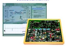
FCL-04 is an advanced digital communication kit designed to perform digital communication experiments using optical fiber as transmission medium for data. It uses 660 nm red visible LED and TTL logic type output photo transistor as optical sensor. Optical link is designed to handle data rate of 512 Kbits/Sec.
