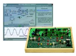
LINK-C is a low cost fiber optics trainer kit designed to perform some basic fiber optic experiments & experimentally measure the speed of light. The phase delay between transmitter and receiver pulse will determine the speed of light through the fiber. A 20MHz dual trace oscilloscope (not included in the kit) is required to make the measurements.
