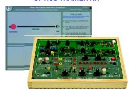
LINK-D is designed to learn basic physics of fiber optics including fiber end preparation. Students can also study the construction of transmitter & receiver to form analog & digital link. Ample number of experiments can be performed with this kit by referring to the exhaustive manuals provided with the kit.
