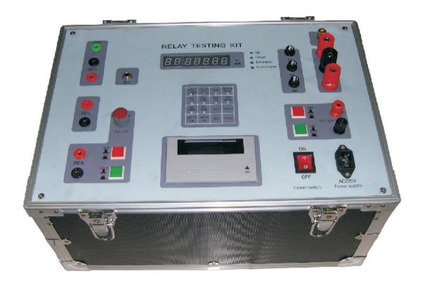
**Introduction:** Model '**DYR-II**' is an ideal, newly developed multifunction relay tester adopting monolithic computer technology. It is composed of auto synchronized digital millisecond timer, logic controlling unit, multifunction digital display, high precision digit collection and processing unit, current-voltage output unit, overload and over range protection unit. Test process is automatic for improved efficiency. The tester has a built in printer for printing the results.
