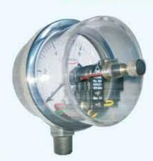
Contact Gauges are ideal in the applications which demands measurement and control of pressure by switching electrical contacts ON and OFF. This eliminates the need of separate switches for pumps and motors which gives audio or visual alarms. The small adjustable magnet mounted in the contact assembly, attracts the contact arm just before the set pressure value which prevent the common problem of arcing and burning of contact pins.
