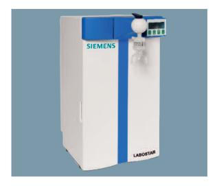
All Labostar systems feature three stages of purification – pretreatment, polishing and a positively charged 0.2µm sterile filter at the point of dispense to provide particle reduction and biological and bacterial protection. LaboStar™ TWF systems also include a 0.2µm vent filter to maintain water quality in the storage tank. LabStar™ TWF systems are available with pre-purification product flow rates of 3 lph and 7 lph for applications with high daily use requirements.
