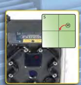
Electronic targets for adjustment of the laser beams to the detector centre.
